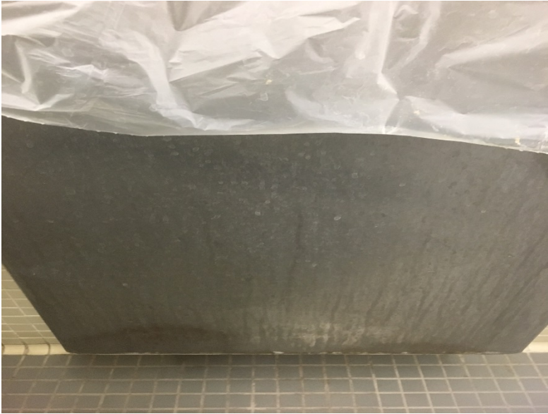
Restroom trash can with heavy water streaking and corrosion
