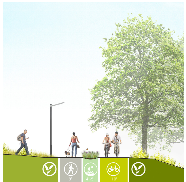
TRANSITION TO WEST HOUSING COURTYARDS WALK 8' STORM WATER PLANTER 4'-5' BIKE PATH (TWO-WAY) 10' PEPPER CANYON
